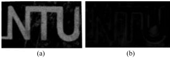
FIGURE 3 The 90° TN cell under crossed polarizers. LC molecules are aligned on the NTU-shaped pattern. (a) The 90° TN cell at the bright state with no applied voltage, and (b) With applied voltage about 3 volts, the TN cell is at dark state due to LCs align vertically with applied electric field.
